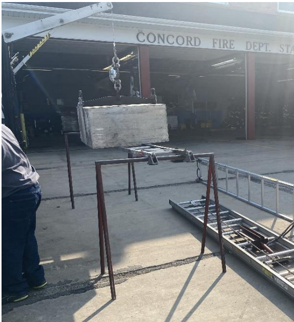
Ladder testing involves supporting 500 pounds for 5 minutes
